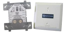
The SSF-FRM1 Addressable Relay Module provides 1 x logical output with 2 x change-over clean-contact outputs for activating a variety of auxiliary devices, such as fans, dampers, control equipment, etc. Compatible for use with 2800 & 3030.
