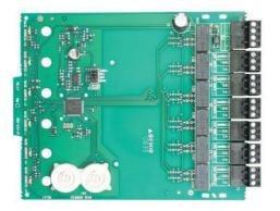
The SS-XP6R is a 6 Relay Control Module for use with the FireSense 2800 & 3030 Series intelligent alarm system.
