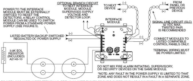
DO NOT LOOP WIRE UNDER TERMINALS. BREAK ALL WIRE RUN TO PROVIDE SUPERVISION OF CONNECTIONS. DETECTORS MUST BE UL LISTED COMPATIBLE WITH MODULE. INSTALL DETECTORS PER MANUFACTURER'S INSTALLATION INSTRUCTIONS
