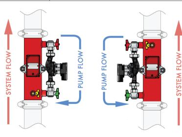
\* As the pump is a recirculation pump, the pump direction is always in the opposite direction to sprinkler flow.
