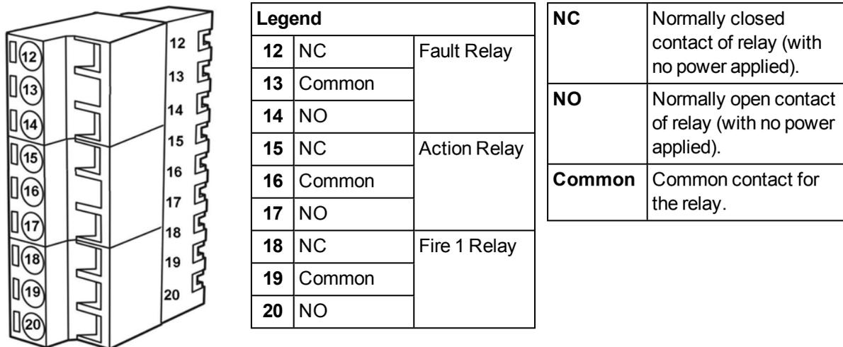
Figure 2-12: Terminal block display, relays
