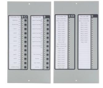
The ACM/AEM-24AT and the ACM/AEM-48A provide a modular line of products for annunciation and control of the AFP-3030 Fire Alarm Control Panel and Network Control Annunciator. The annunciators provide an array of LEDs to indicate point status and, in some versions, switches to control the state of outputs or zone disablement. These annunciators use a serial interface and may be located at distances of up to 1,800 metres from the panel.
