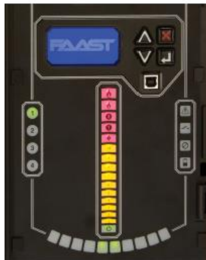
User Interface Display: Intelligent FAAST XT and Intelligent FAAST XT PRO
