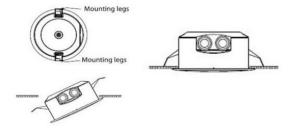
(Note: the spring tension clamps are suitable for ceilings which have a thickness of 9mm to 25mm and are fitted with rubber boots to reduce soft ceiling tile damage. Ceilings which use a perforated steel grill type panel (less than 5mm) may require extra backing support to increase spring tension and reduce the risk of speaker sag over time).
