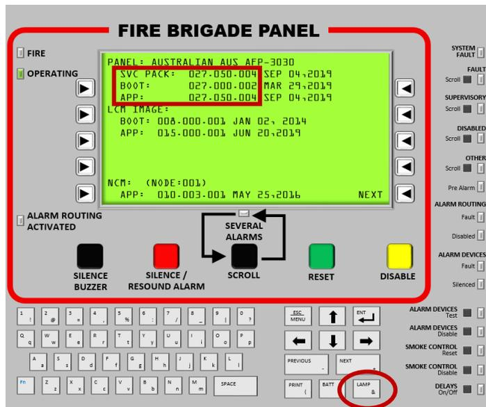
**Step 8** The current firmware in the panel should be 27.50.
