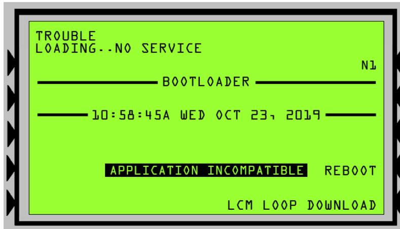
**NOTE: For 3030 CPU's without a display, the fault 'N# Loading – No Service...' will be present on the NCA.**
