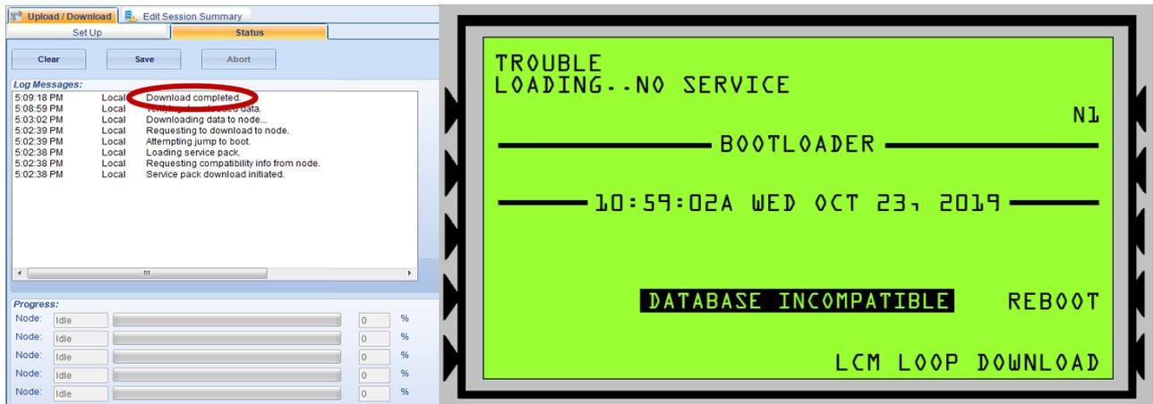
**NOTE:** For CPU's without a display, the fault 'N# Loading – No Service...' will be present on the NCA. Wait until the node appears in the online session in VeriFire Tools before proceeding.
