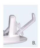
The "Rat-Trap" utilises a spring latching system. Each latch is set like a rat trap before installation into the speaker hole (A.). When the speaker is pushed into the ceiling, the latches spring open, securing the speaker in place (B.).
