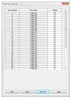
**Note:** Tube flow scan is only available in VEA firmware 5.30 or above, for previous firmware Flow Scan is the only mechanism available to do the flow measurement.
