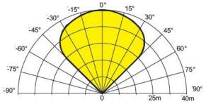
To meet the requirements of EN54:10 clause 5.4, where the ratio of the response points Dmax: Dmin should not exceed 1.41, the horizontal and vertical viewing angles max should not exceed ±30°.
