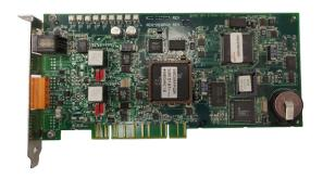
While embedded gateways have IP capability and connected via a Cat-5 cable, the ONYXWorks® PC Gateway alternative is connected directly to the NFN, whether it be through wire, low-speed multimode fibre or high-speed singlemode fibre. The version of PC card needed will depend on the type of connection overall.
