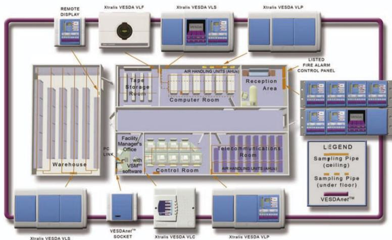
Having all VESDA smoke detectors on a VESDAnet loop allows you to configure and interrogate each detector from a central location, in this case the Facility Manager's office.
