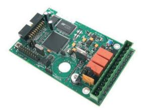
The VESDA VLF MCC (Multi-function Control Card) is an interface card for the range of Xtralis VESDA VLF smoke detectors. An MCC expands the range of input and output communications a VLF detector can perform.
