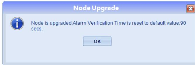
**Step 12** Perform this process for each node that is being upgraded. Each node's database version should indicate that it is now V28.
