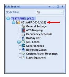
Now that the configuration(s) have been upgraded and a backup has been saved, the firmware can be downloaded into each node [either individually (via 3030/NCA2) or simultaneously by doing a Distributed Download (via the network card)]
