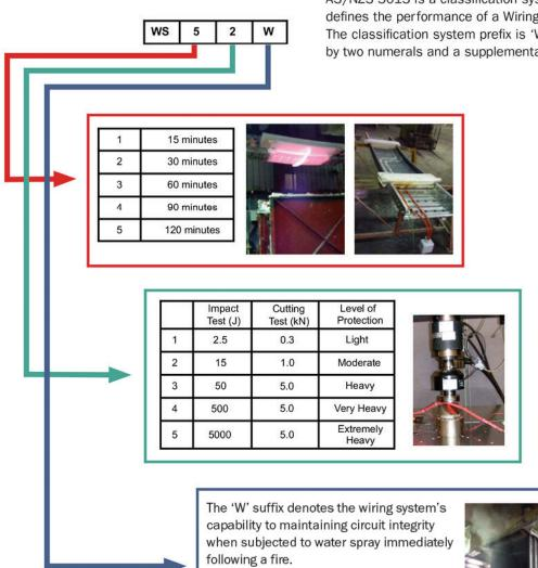
Cables are subjected to fire at 1050°C for 120 minutes, then water sprayed for a
